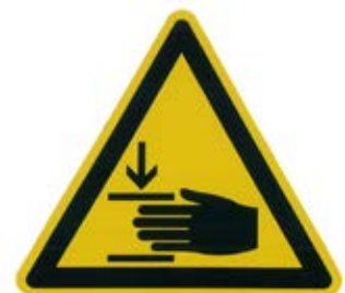
Fig. 4: Warning sign PN 671640-1 Pay attention: Do not place your hands between moving parts.
