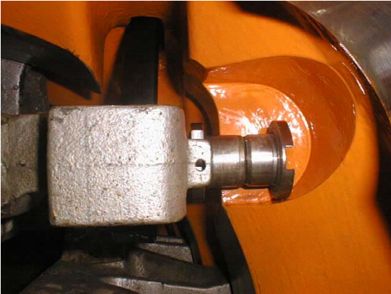
Figure 6 Retainer pin is pulled out
