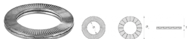
Fig. 75: Nord Lock Washer detailed illustration
