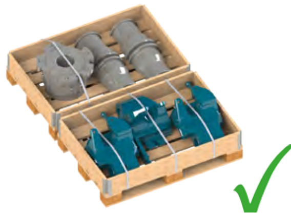
Fig. 167: Correct Storage on pallet boxes
