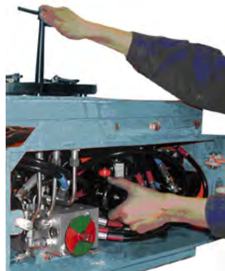
Fig. 56: VES SD 750 - Moving the trigger
