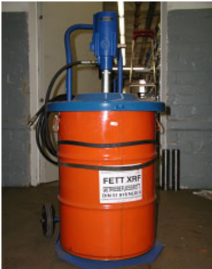
Grease Pump (Part No. 775810)
