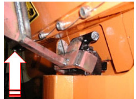
Fig. 03: Cover Assembly unlocked: Press Unlock Tool inwards
