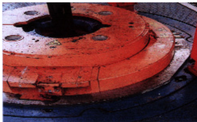
B+V PS750-2/1000 installed in the rotary table
