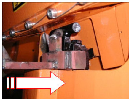
Fig. 02: Cover Assembly locked
