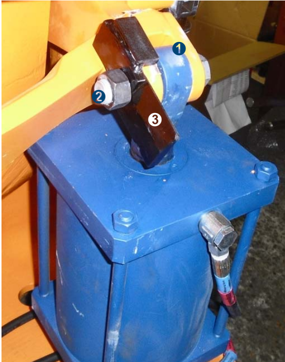
Figure 13 Cylinder eye with Signal bar for Feedback Valve
