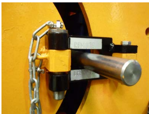
Figure 22 Break handle and fork position during remote operation
