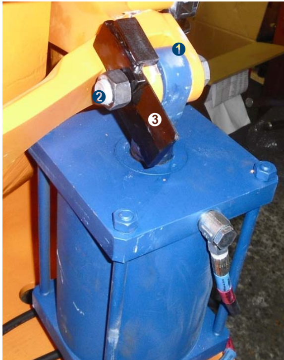
Figure 4 Cylinder eye with Signal bar for Feedback Valve
