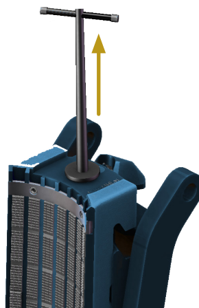
Fig. 83: Lift carrier out with Crane on Lifting Tool
