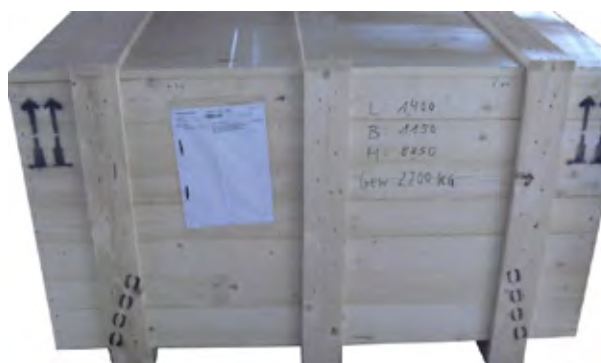
Fig. 22: Typical transport and conservation packing for PS 350
