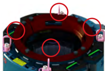
Fig. 25: Hoisting eyes on upper ring
