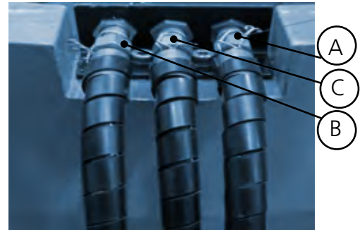
Fig. 9: Hydraulic Connections on Side of Body
