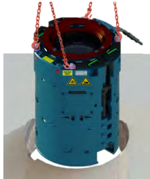
Fig. 36: PS 350 removal from Rotary Table
