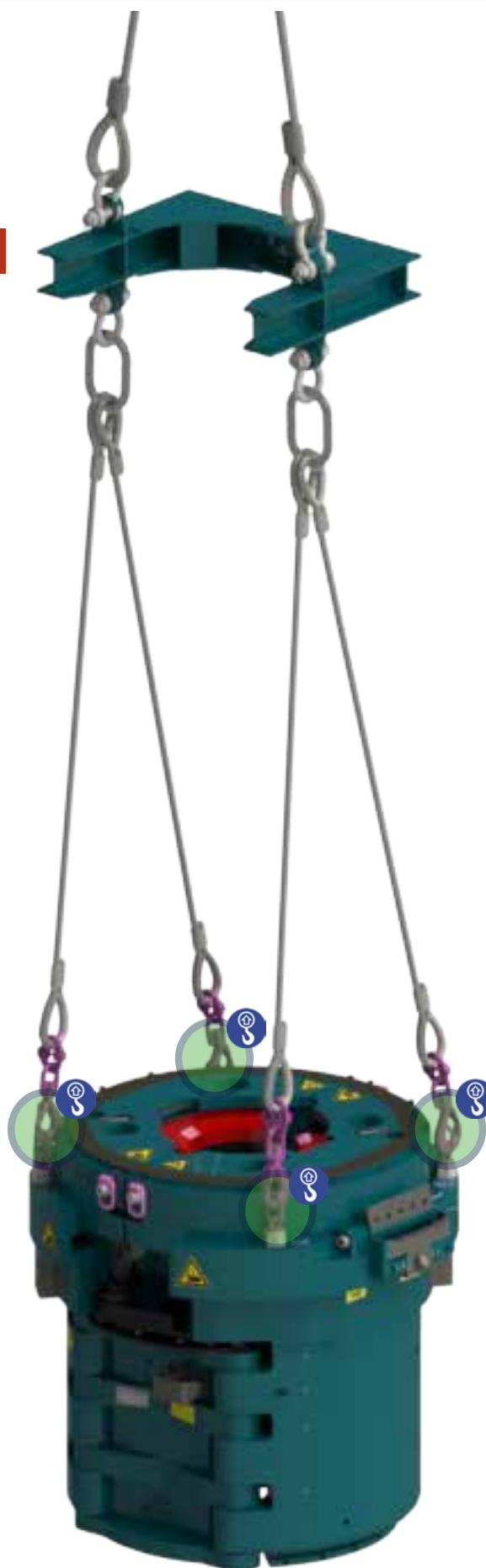
Fig. 58: PS-500 attached to Lift Beam Assembly
