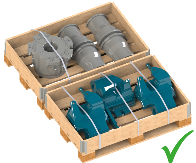
Fig. 42: Correct Storage on pallet and pallet borders
