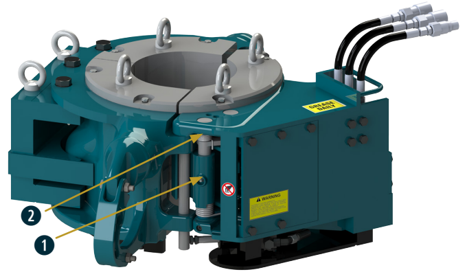
Fig. 34: Lubrication points I
