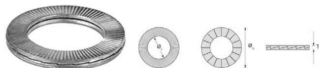
Fig. 51: Wedge-Locking Washer detailed illustration
