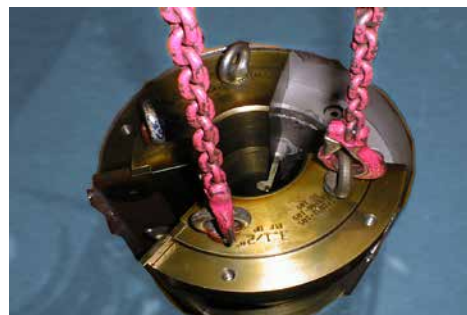
Fig. 36: Remove bushing VES SDS
