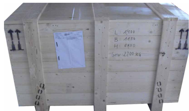
Fig. 32: Typical transport and conservation packing for SDS
