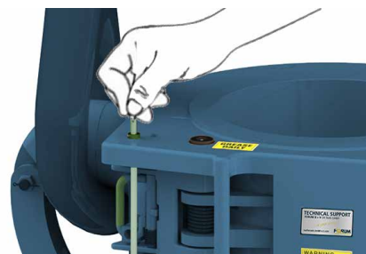
Fig. 49: Check PIN seat
