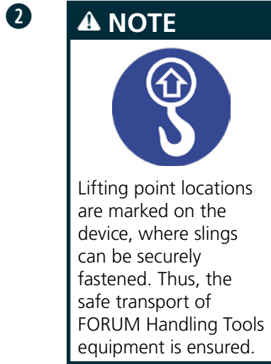
Fig. 24: Lifting point ANSI Z535.4 PN 671639
