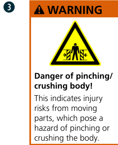
Fig. 25: WARNING sign "Body crushing" ANSI Z535.4 PN 671641
