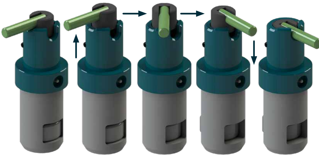
Fig. 37: Slip Lifter - Locking Pin sequence
